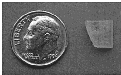
Figure 1. Single crystal of [(C 4 H 9 ) 4 N] 3 (V 3 O 9 )·0.5H 2 O shown with a dime for scale.
